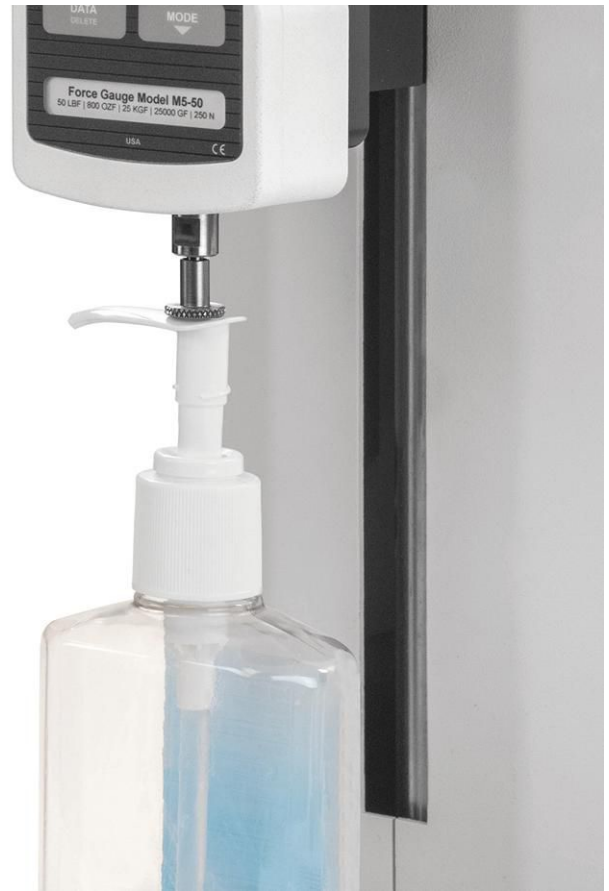
A sanitizer pump dispenser is tested in compression.
