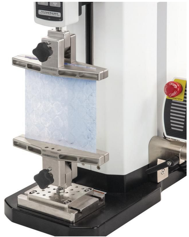
A tensile test is performed on a disinfecting wipe.
