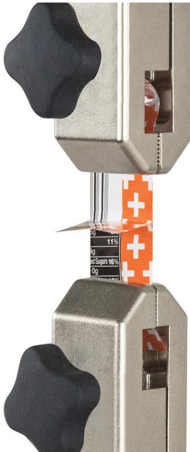
An example of peel testing with manual grips.
