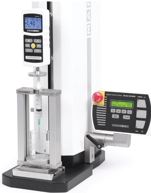
A syringe is tested to determine plunger force activation.
