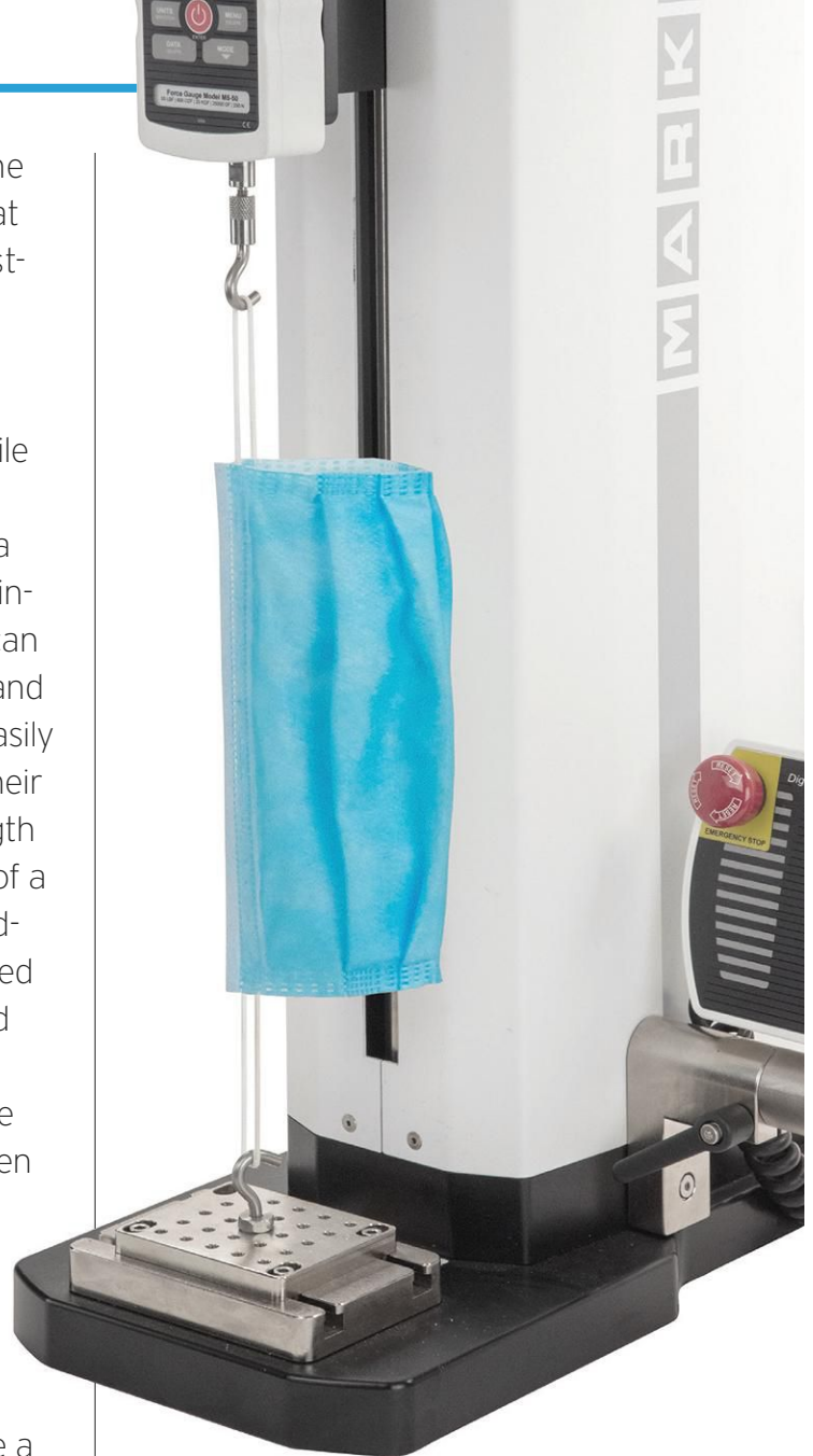
A medical-grade surgical mask is tested using hooks.
