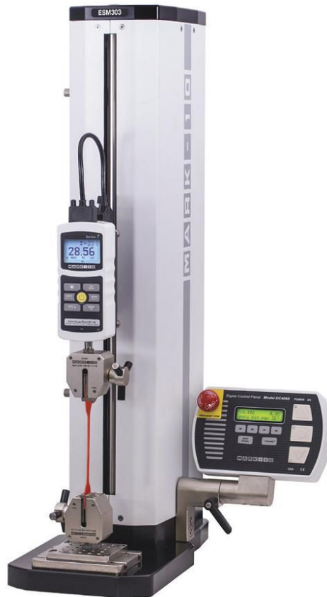
This small, benchtop tensile tester is rated to 1.5 kN, and may be used for tension and compression applications. The unit is shown with a force gage, which integrates a load cell and indicator into a single housing. Source: Mark-10
