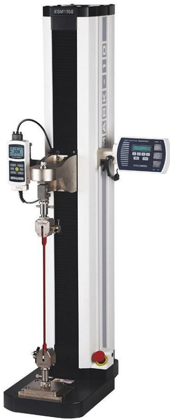
A 6.7 kN tensile tester is shown configured for an elastomeric tensile test. The sample is secured between two wedge-action grips. Force and travel distance are recorded and output to a PC for further analysis. Source: Mark-10
