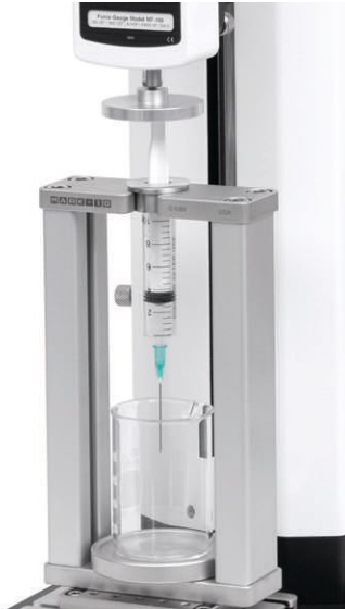
The resistance force of a syringe's plunger can be measured by a compression force tester. Source: Mark-10
