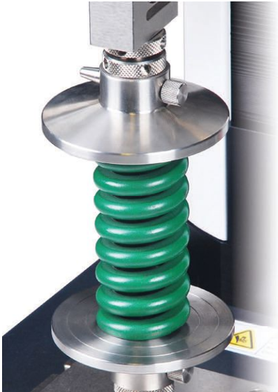
Spring rate can be determined by compressing a spring to one or more heights and measuring the corresponding forces. Source: Mark-10
