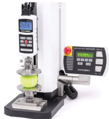
A typical compression force testing system consists of a test stand, force gage, and application-specific grips and fixtures. Many compression testers are capable of tension measurement as well. Source: Mark-10
