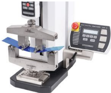
A 4-point bend test performed on a plastic sample helps shed light on its performance characteristics while preserving its integrity. Source: Mark-10
