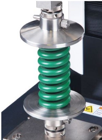
A compression test is performed on a spring. Source: Mark-10
