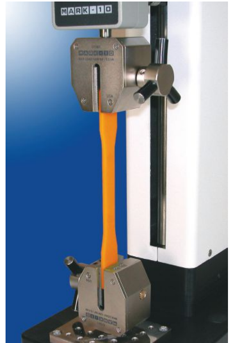
Force measurement systems can be used for basic tensile testing of relatively elastic materials, while materials testers are better suited for stiffer samples. Source: Mark-10
