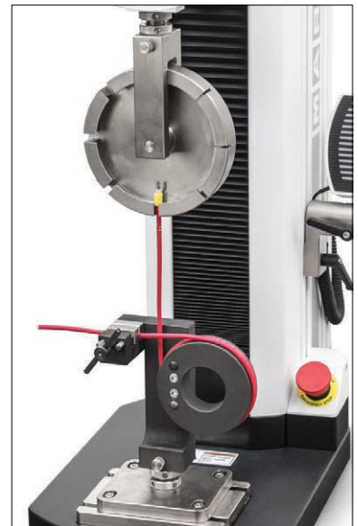
A wire terminal test is performed with a turret-style grip and a ballast-style grip.
