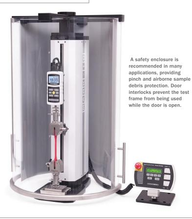
and lowered risk of overload, it's recommended to use a load cell between 10% and 90% of its range. Load cells often have mechanical overload protection to 200% of the published range, but it is still not recommended to exceed 100%.
