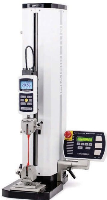
A force measurement testing machine is shown with a pair of wedge-action grips. The machine's preload function zeroes out the force offset produced by the "first bite" of the spring-loaded grip jaws. Source: Mark-10
