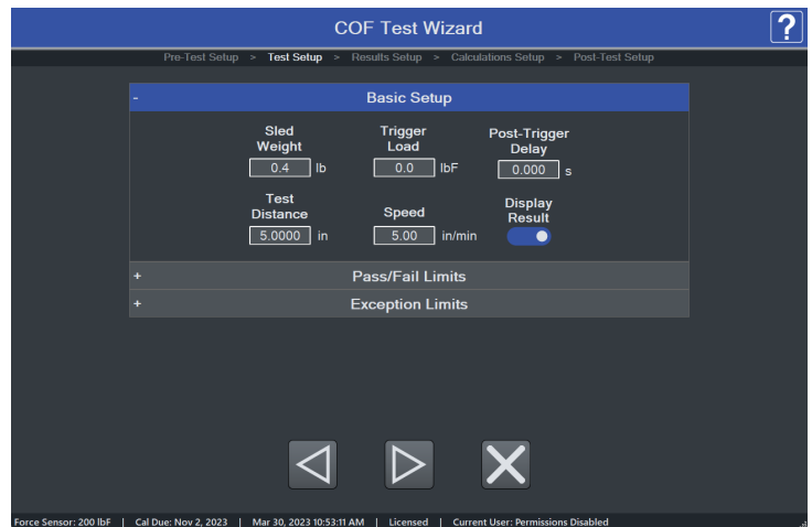
Specify sled weight and data collection start and stop triggers during test setup.
