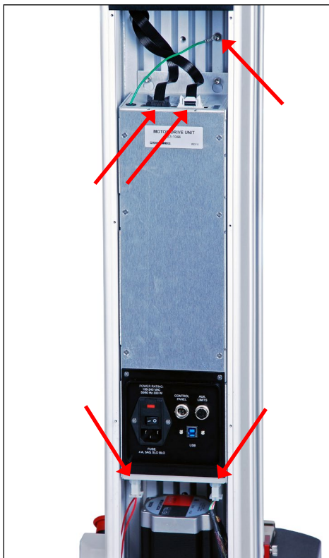
Locations of connectors and ground wire
