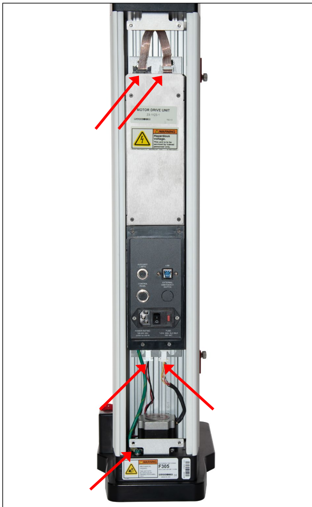
Locations of connectors, ground wire, and bracket
