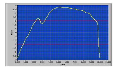
MESURgauge Plus plots load versus time or load versus travel, depending on the system configuration. X-axis and Y-axis minimum and maximum values can be changed by double-clicking on the numerals along the axes. When the numeral is highlighted, type the desired value, then press **ENTER** or click away from the area.
