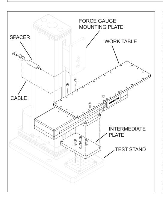
The G1045 90° peel fixture mounts to the base of a compatible Mark-10 test stand. The illustration at left depicts proper assembly. Please follow these instructions:
