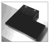
To mount a force gauge, it is necessary to temporarily remove the gauge adapter from the crosshead. Loosen the two 5/16 screws (shown at left) using the included tool kit. Then, mount the gauge to the adapter using the four included gauge mounting screws. After the gauge is mounted to the adapter, mount the adapter back onto the crosshead with the 5/16 screws.
