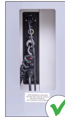
Fig. 3 Proper cable routing
