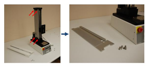
4. Remove the limit switch support plate by loosening the four Allen screws, as shown below:
