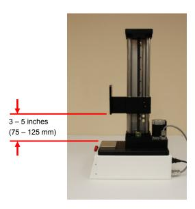
13. Before re-installing the limit switch support plate, be sure to position the limit switches at their furthest allowable extremes, as shown below:
