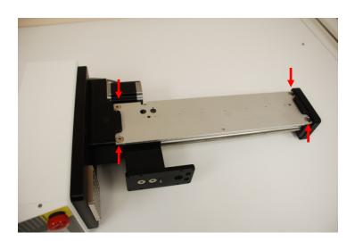
11. Install the encoder with the three supplied screws (two flat screws, one Phillips screw), through the clearance holes in the support plate, as shown below:
