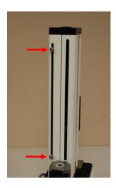
2. Remove both sheet metal covers from the test stand by loosening the four screws on each side, as shown below:
