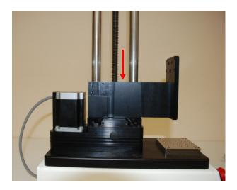
Position the test stand on its right side. 6.
