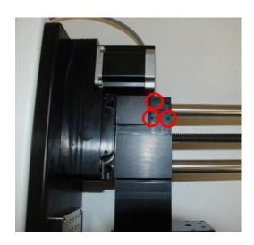
8. Position the linear encoder on the linear displacement strip, at the end of the support plate, as shown below:
