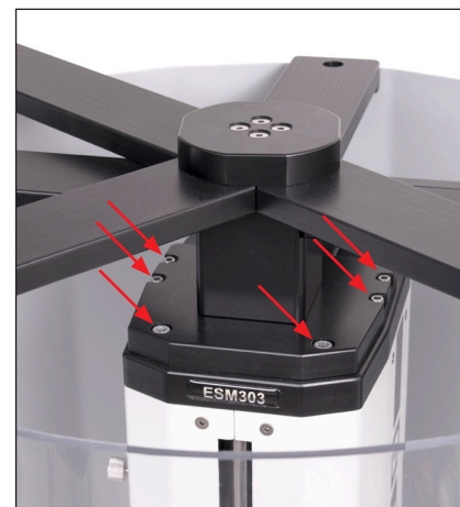
Fig. 1 Attaching the shield assembly to the top of the column
