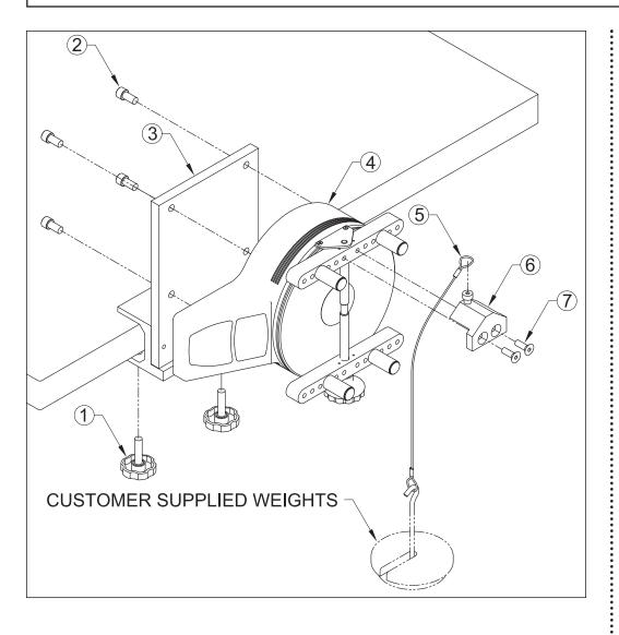
The AC1036 calibration kit is designed to permit the field calibration of any Series TT01 cap torque tester. The kit contains a complete set of attachments required to mount the tester to a bench, as well as the necessary brackets and cable to mount weights. Please note: weights are not available from Mark-10, and must be supplied by the user. The illustration at left depicts proper assembly. Please follow these instructions:
