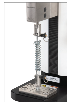
Tension spring testing
