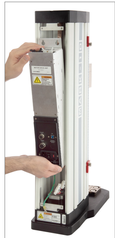
Removing the electronics module
