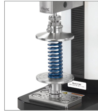
Compression spring testing
