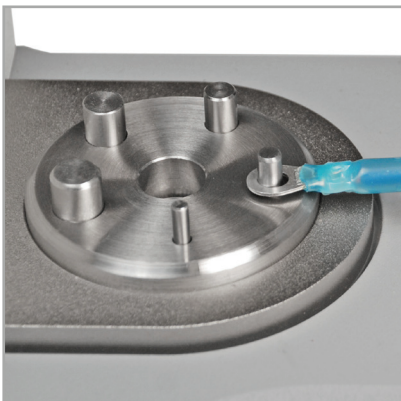
WT3002 Ring terminal fixture
