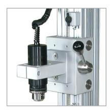
A Series R50 torque sensor is shown mounted to a model TSTM-DC motorized torque test stand. The sensor fits into the stand without the need for additional adapters.
