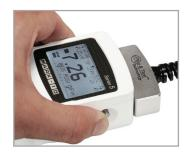
Included certificate of calibration contains 10 data points in each measuring direction. A combined certificate for the sensor and an indicator is available at time of order, part no. CERT-SI.
