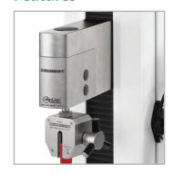
Series FS05 sensor is shown mounted to the crosshead of an F305 test frame, configured for a tensile test.
