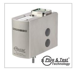
Series FS05 force sensors measure tension and compression force, and are designed for use with Series F test frames. Capacities available from 0.12 to 500 lbF [0.5 N to 2.5 kN]. Also compatible with Mark-10 indicators (sold separately) through unique Plug & Test® technology. Includes a certificate of calibration with data.
